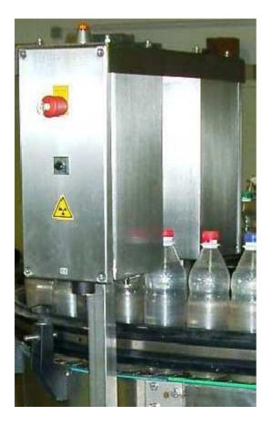
Oher influences that create problems for other inspection methods i.e. foil, do not have any effect on the X-ray measurements.
